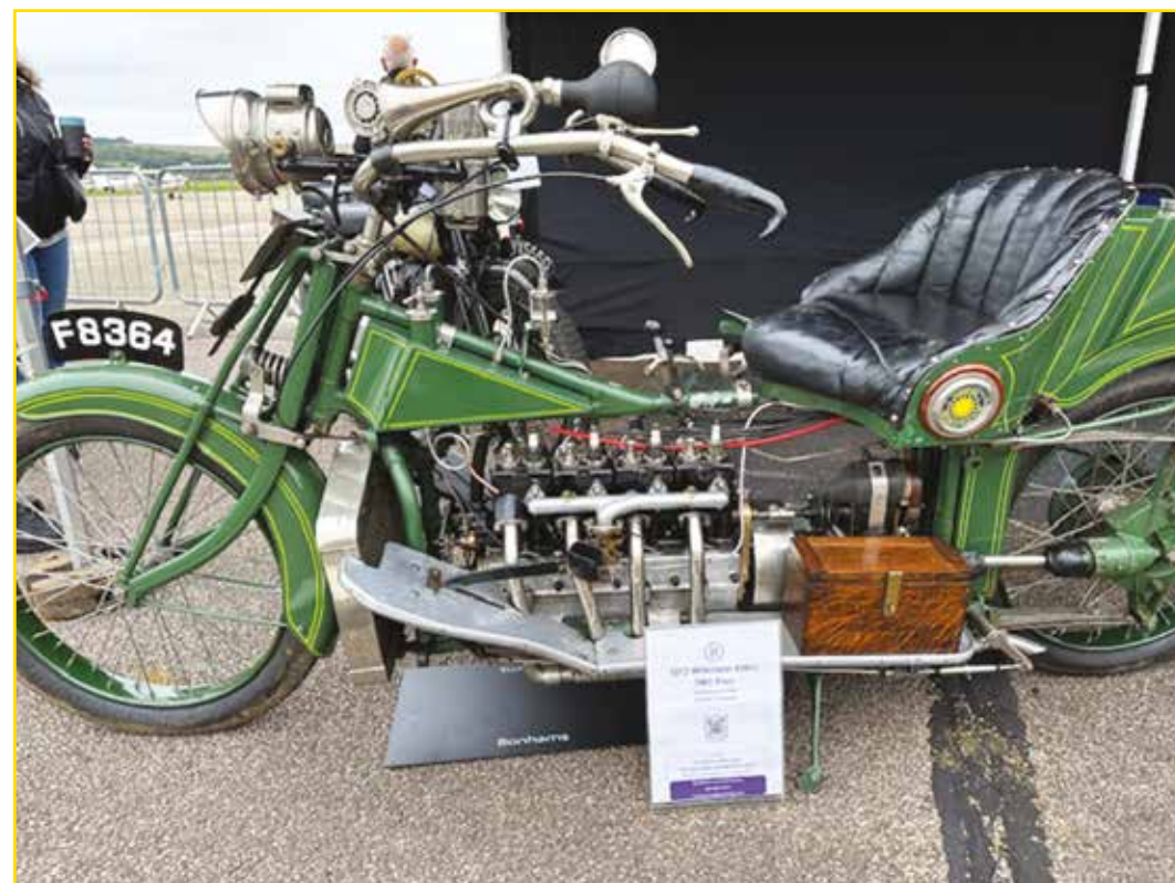
An early Gold Wing? A 1913 Wilkinson (yes the razor blade people). 4 cylinder, 800cc, shaft drive, rear suspension by leaf springs, seat by Harrods? 65mph and no front brake!
