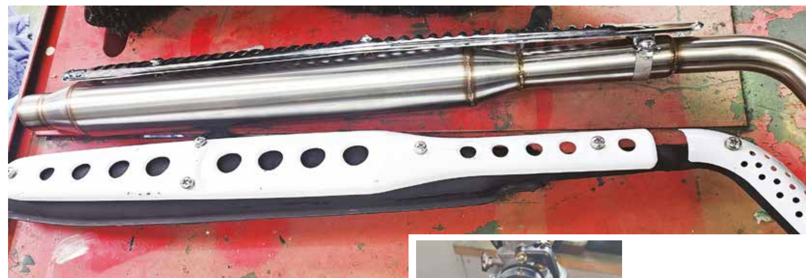
Big bore stainless steel pipe at the top. Standard pipe below.
