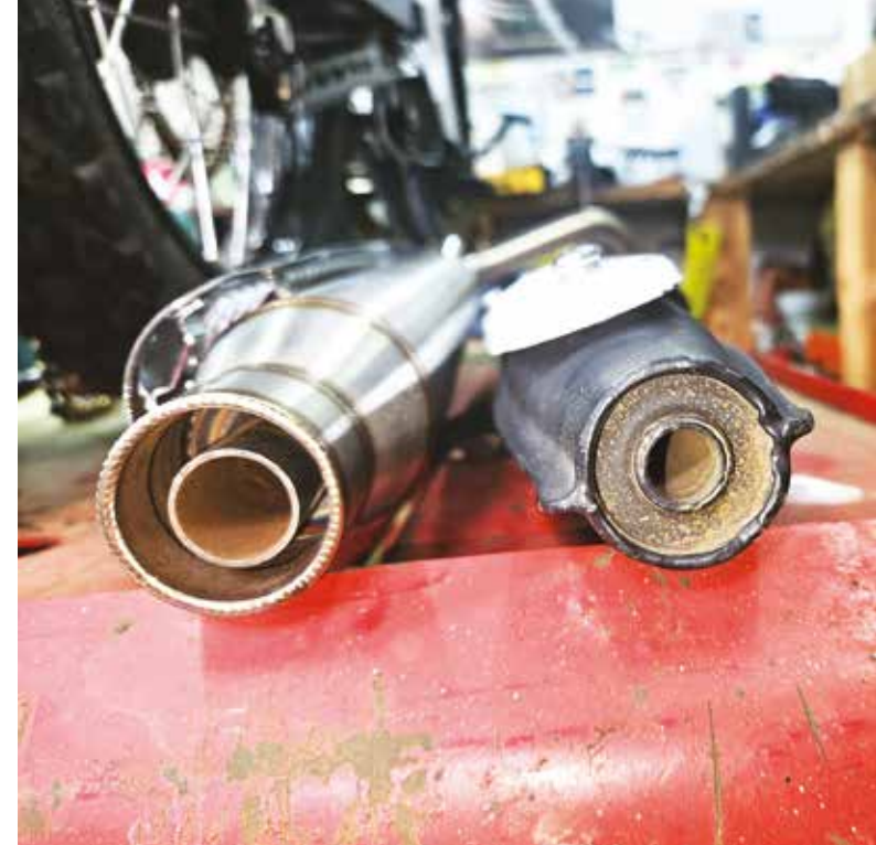
The bigger bore exhaust pipe on the left
