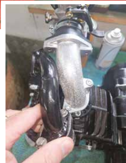
The carb manifold. The new big bore is on the right.
