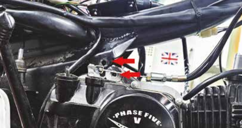
These two holes should be in alignment
