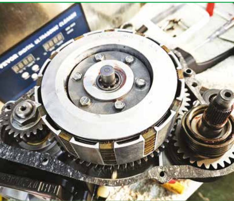
Clutch basket fully loaded with oily plates
