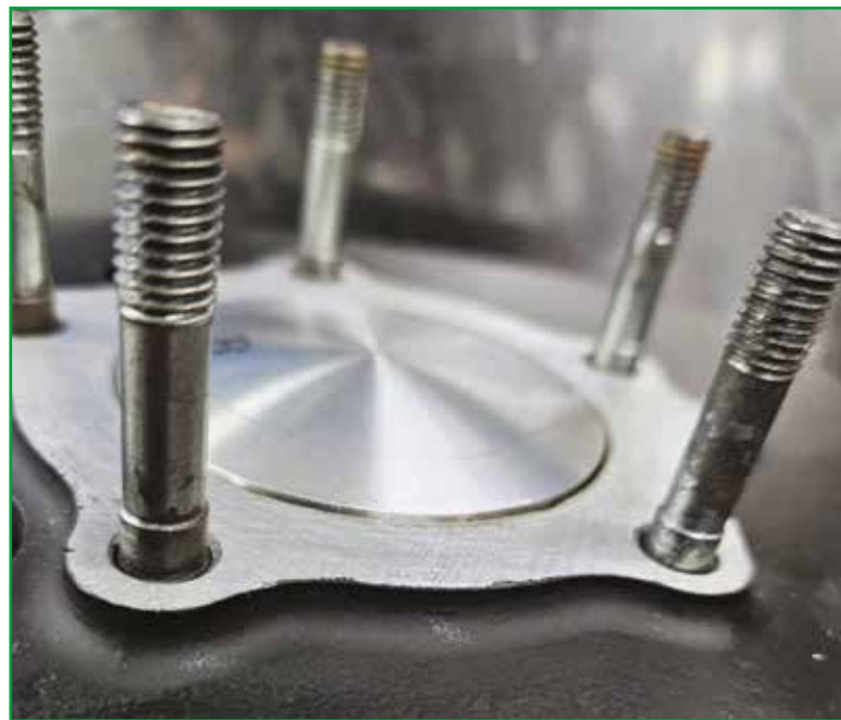
"The piston was just poking up a smidge too far."
