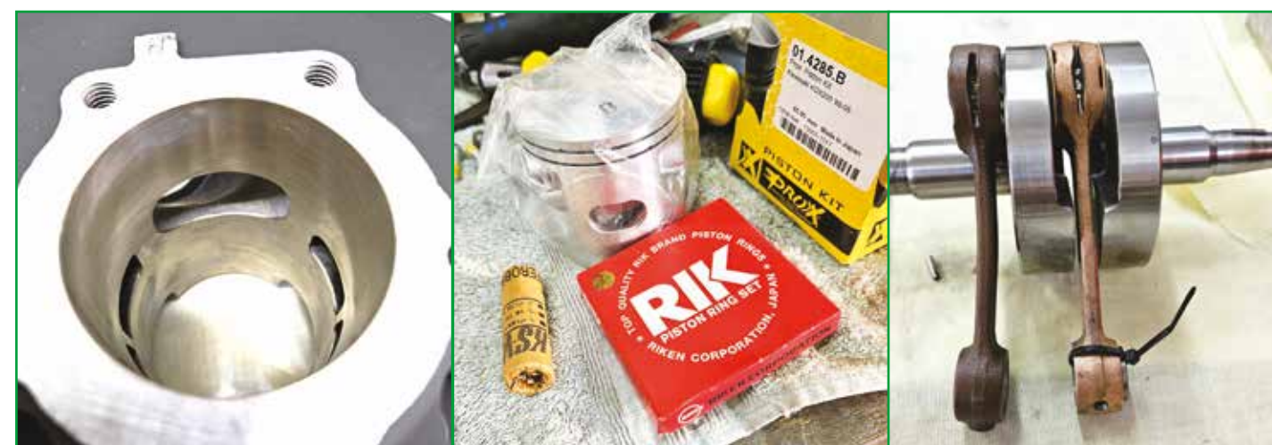
The re-Nikasil-plated bore is better than new
