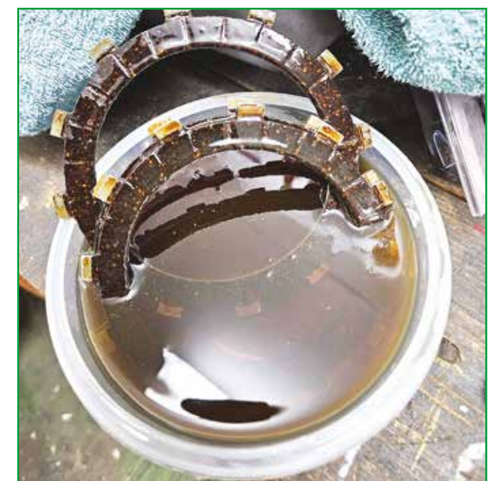
Clutch plates soaking in oil overnight
