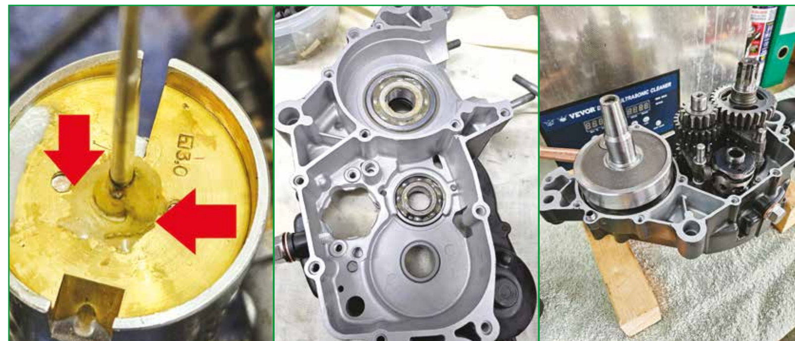
"The previous owner had had a significant issue with the carb. . ." which he had tried to repair with a big blob of glue!
