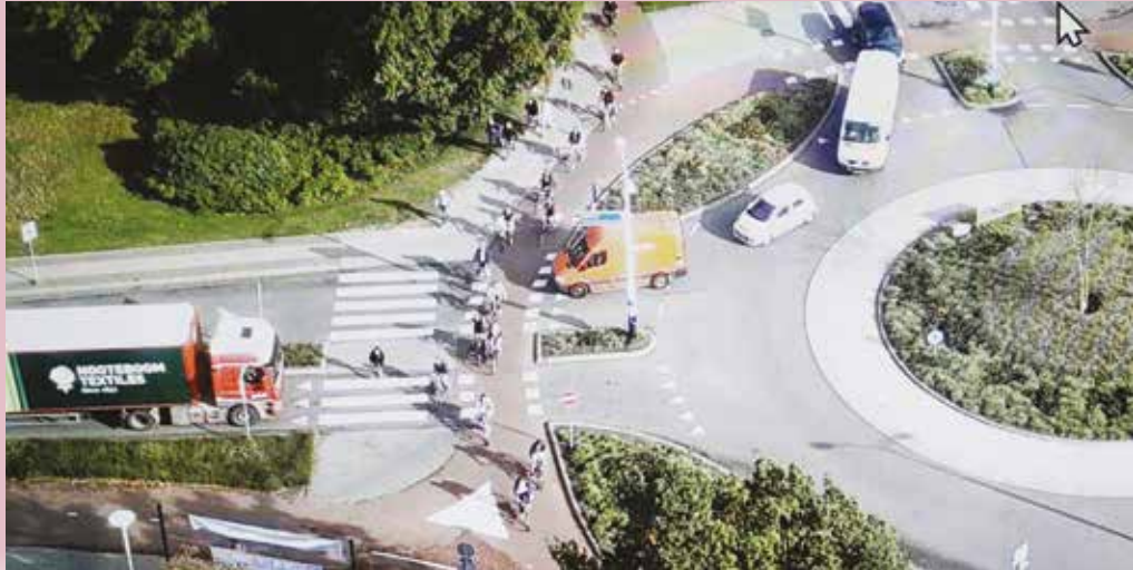
A Dutch style roundabout. It is a very small roundabout and the vehicular traffic is very light, yet it took the lorry 1 minute 37 seconds to enter the roundabout and leave. Think what would happen if every car at every roundabout took, say, one minute to enter the roundabout.
