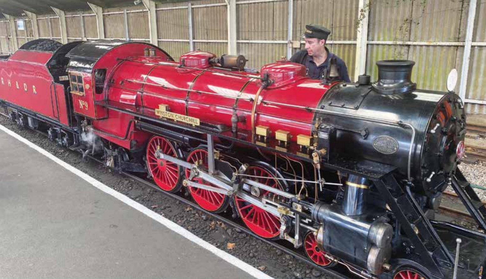
The Winston Churchill, a 4-6-2 Pacific locomotive built for the RH&DR in 1931!
