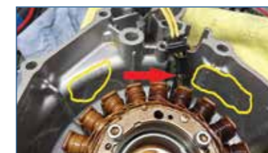
This is when that little part that was highlighted earlier, came to haunt me. Here I have removed it but you can see it was starting to damage the stator wiring (arrowed) and the inside of the case (circled).
