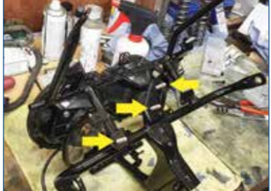
Here is a good example of a sub-project. I've cleaned the lights, rubbers and fasteners and started rebuilding the headlight assembly. This is a small project that you can work on, complete, and put to one side when done. You can see where threads were blasted but then masked before being powder coated on this assembly.
