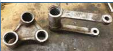
The suspension linkages, also now bearing free, but this was also a tough job and a lot of heat from a gas torch and a good amount of swearing proved to be (literally) pivotal here.
