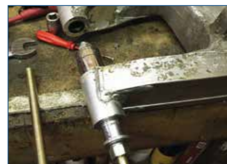
Extracting the suspension bearings was probably the toughest part of the whole rebuild. These things really did not want to move after 30 years.
