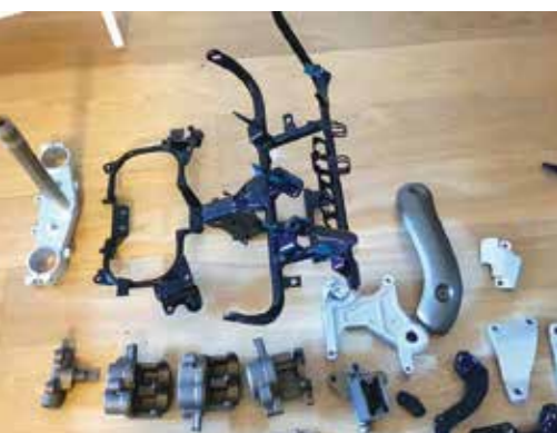
Various parts after coating. The black parts are powder coated, while everything else is Cerakoted, either in silver or a bronze colour
