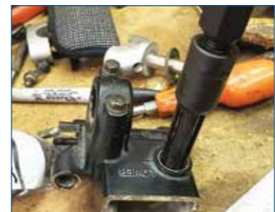
Actually, the glass itself came out easily, but there was a metal frame remaining and here I'm using a bearing puller to remove that.
