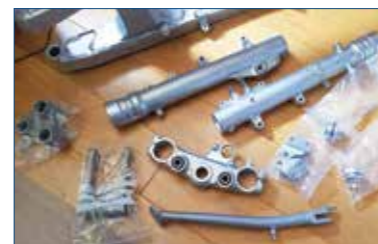
Once bearing free, the forks and various suspension parts were sent off to Dave at 'TSR Vapour Blasting Services' in Sevenoaks before they were powder coated or Cerakoted or just painted.
