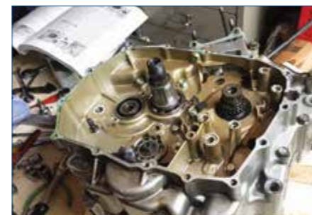
It was then a case of evenly undoing the multitude of bolts that hold the engine cases together and finally using specific levering points to ease the cases apart.
