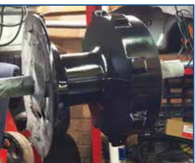
The rear hub. Cleaned, flatted down, etch-primed and painted satin black.
