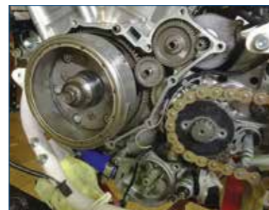
This shows the left side of the engine, where you can see the starter motor at the top, the rotor for charging and ignition timing and one half of the water pump at the bottom. The gasket surfaces are spotless and awaiting a new gasket and the cover.
