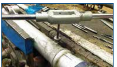
Tapping for the Helicoil
