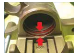
Here you can see the two seal grooves. The deeper one is the hydraulic seal, the outer one the dust seal. These are the front calipers with the seals in place.
