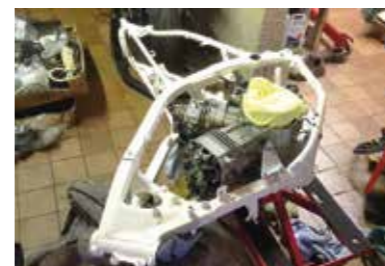
With the engine on its side, the newly powder coated frame was lowered over it, an idea that worked pretty well without damaging the fresh paint.
