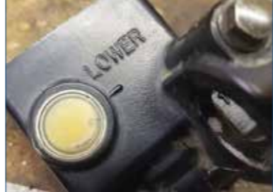
This was the front master cylinder. The sight glass really wasn't much use. Luckily, replacements are available from China via Amazon. The trick was getting the old glass out.
