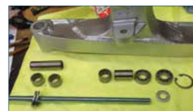
My home brewed 'bearing installing kit'. Just add suitably sized sockets and threaded bar
