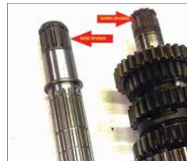
Note the difference between the new and the worn splines.
