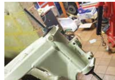
New head bearing races were pressed into the headstock...
