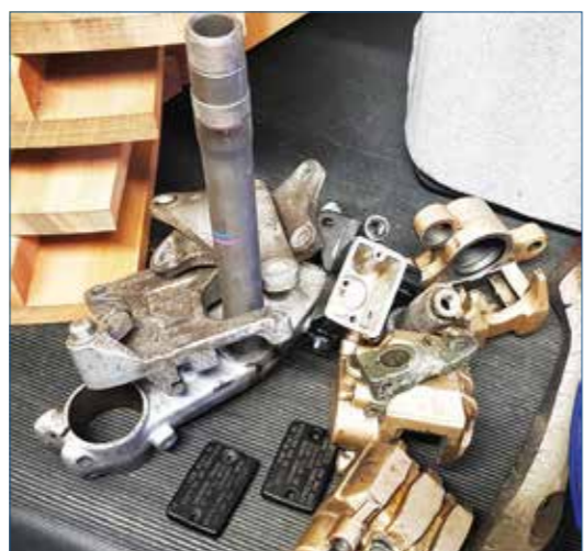
A picture of what I took to be Cerakoted. These are brake calipers, master cylinders, various brackets and fork lower triple clamp with the bearing race removed.
