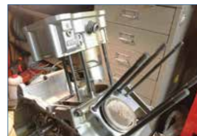
Once the case halves are back together, along with new O rings for the oil pump, it's time to clean up the mating surfaces, the barrels and the engine cases, fit new barrel gaskets and lower the barrels on to the engine, carefully persuading the piston rings into the bores.
