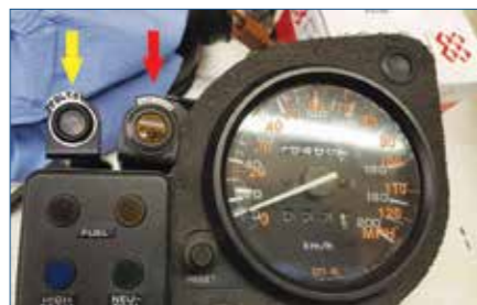
Voltage indicator on the instrument panel beside the 'official' Honda 'afterthought' side stand switch
