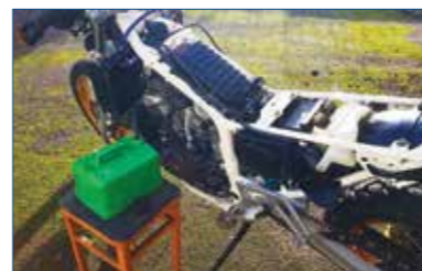
And with a temporary fuel supply to see if she will start.
