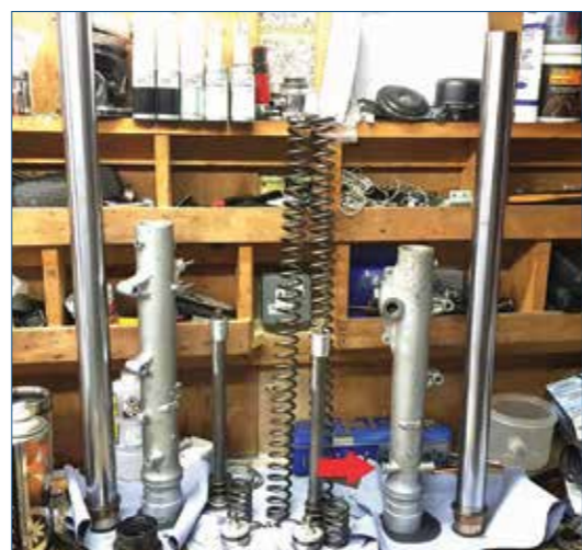
The forks were another sub-project. I have no idea when the fork oil had been changed. But from the look of it 'never' would be a reasonable guess. It was a green colour.
