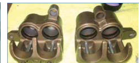
And with the help of hydraulic fluid, the pistons are now in place, along with a few other rubber components. Another little project done.
