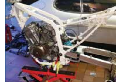
... and more new and reconditioned parts were fitted to the frame. Here the swing arm, suspension links and the shiny new Nitron shock are all in place...
