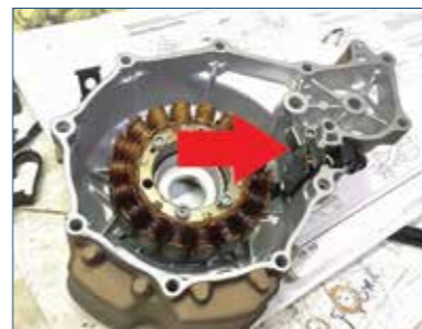
Here is the side cover with the stator. There is a small plate held on by a cap head screw at around the 3 o'clock position. This simple little part would come back to haunt me.
