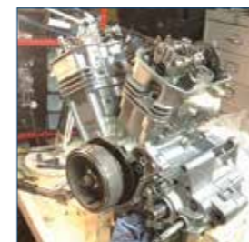
Here the heads are back on, and the camshafts and cam timing chains are in. Note the engine's paint finish, which is original and 32 years old. It has held up really well.
