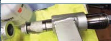
Here the bar and nuts with suitable sockets are being used to press the bearing in. The masking tape on the socket gives me an indication of when the bearing is fully seated.
