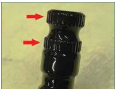
What not to do. This is the splined end of the rear brake pedal. It's a very precise fit into an actuating arm. The splines should have been masked before powder coating. If this had been Cerakoted, it would have been fine. This powder coating had to be blasted off and the part was then re-powdered after masking.
