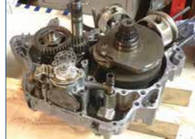
Finally, we are there. Crankcase split. The large gear on the left side of the engine is one of the gearbox gears and is at the top of the output shaft, so that has to come out. You can also see the crank, counterweights and pistons clearly here.
