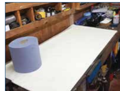
This is where the patient will be laid out. The surface is hardboard coated with sticky back plastic to give a cleanable surface. It won't last long, but long enough.
