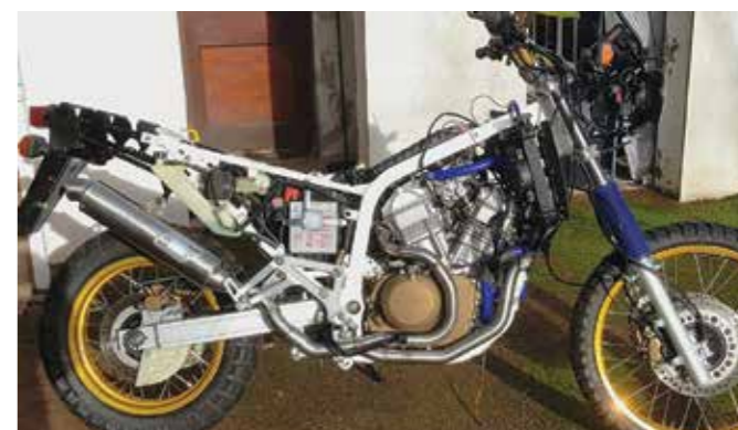
New wheels with new Mitas E07+ tyres and she starts to look like a bike again. The wheels have the discs mounted and the calipers fitted, along with a new rear sprocket, and a shiny new chain. Other parts that were reconditioned were the two radiators at the front, along with the radiator mount. These were vapour blasted and then painted at home with heat-resistant radiator paint.
