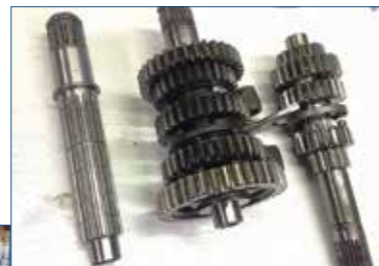
Here we have the components of the gearbox. All the gears have to be carefully removed from the old output shaft and assembled on the new shaft, on the left.
