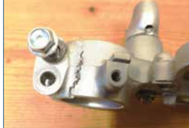
... and bang, the top yoke broke.
