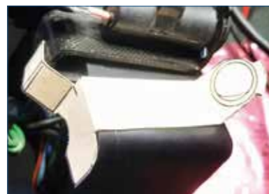
I made a cardboard template of a bracket that apes the Honda side stand switch on the instrument panel.
