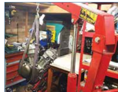
While I could just about lift the engine, it was silly to risk hurting myself, so I drafted the engine crane into action.
