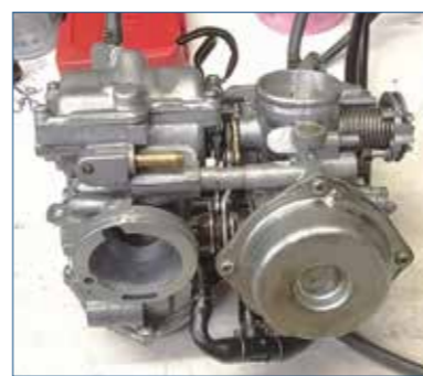
The cleaned and rebuilt carbs, with new seals and replacement needle valves that had worn.
