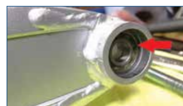
A bearing with its circlip in place. A dust seal will go in next.
