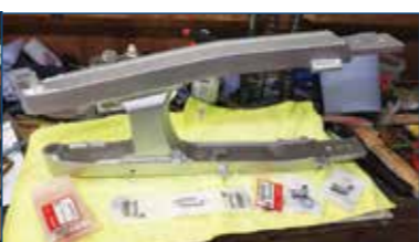
Although it looks the same as it did before, the swing arm has here been Cerakoted and awaits its nice new bearings.
