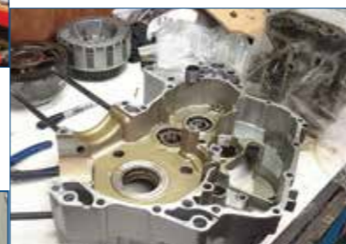
There is no gasket between the two case halves, so 'Hondabond' sealant is used. Before assembly, the mating surfaces need to be spotless and cleaned of all the old sealant. A time-consuming job using sharp blades and acetone.
