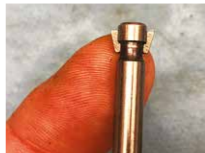
Left: Exhaust valve with tiny, tiny collets Above: Tiny collet, big finger
