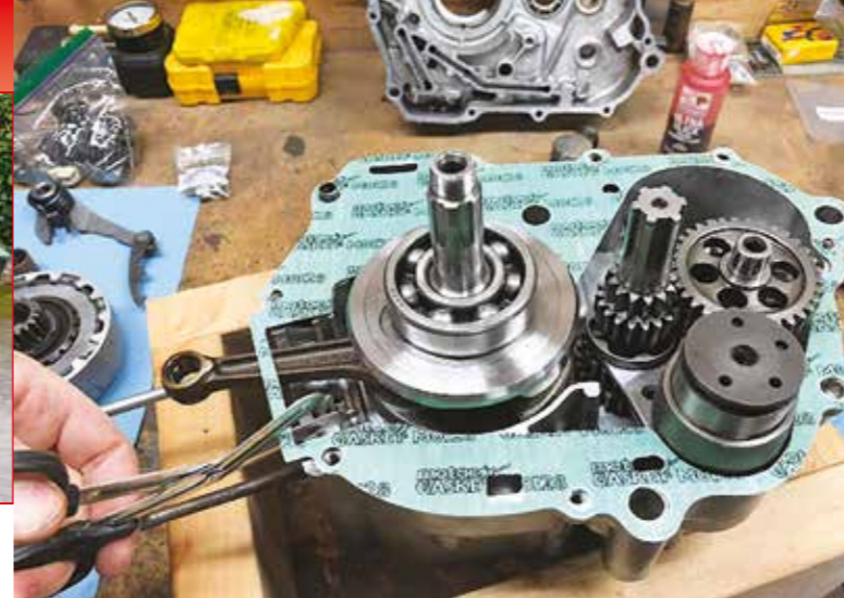
Left side crankcase with crankshaft and transmission in place.
