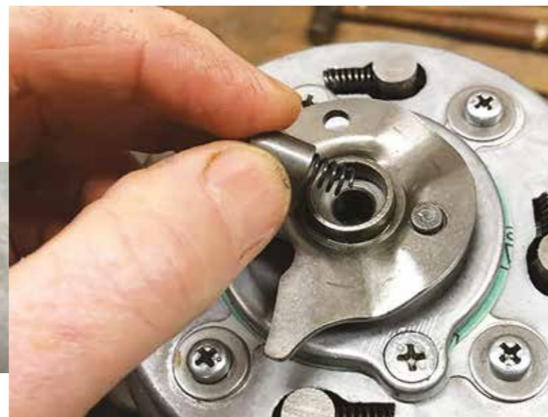
"... pesky oil feed pipe with the spring being installed the correct way."
