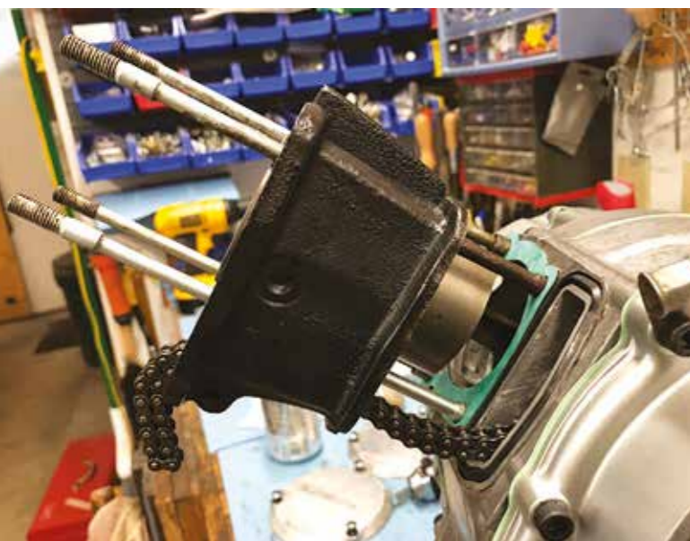
Left. Cylinder being installed Above. Ensuring that the just visible 'O' is at top dead centre Below. Finished
