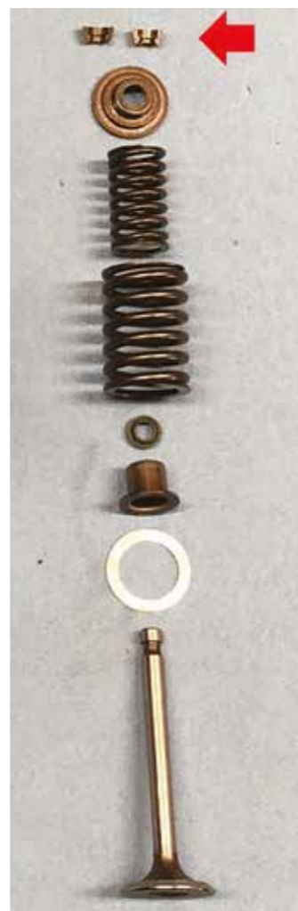
Left: Exhaust valve with tiny, tiny collets Above: Tiny collet, big finger
