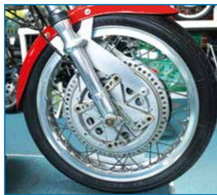
More museum sculpture. I know it’s just a front brake, but imagine designing something that functional and that beautiful. This is the state-of-the-art Fontana brake as fitted to the 500 Linto racer of 1969. Such talent. We may have better brakes today, but they are ugly lumpy things; they work but they don’t look like this. When you wanted to stop on a racing bike in the sixties you needed big brakes. Virtually all road bikes of the time had simple single-leading-shoe brakes. Racing bikes usually had twin-leading-shoes, but the Fontana had four leading-shoes. Imagine the pull on the brake lever that needed.
