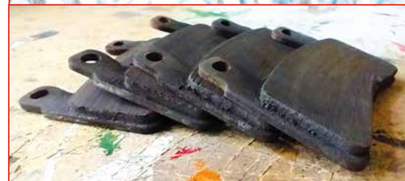
The old front and back Kyoto and Goldfren disc pads still with plenty of wear after 6000 miles and four track days.
