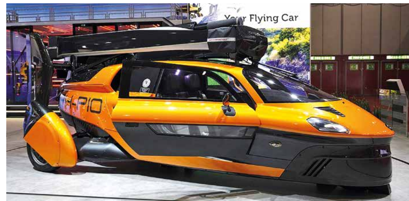
The PAL V is available now. It is a gyrocopter and can fly and drive at 100+mph. Take off run is less than 100yds.
