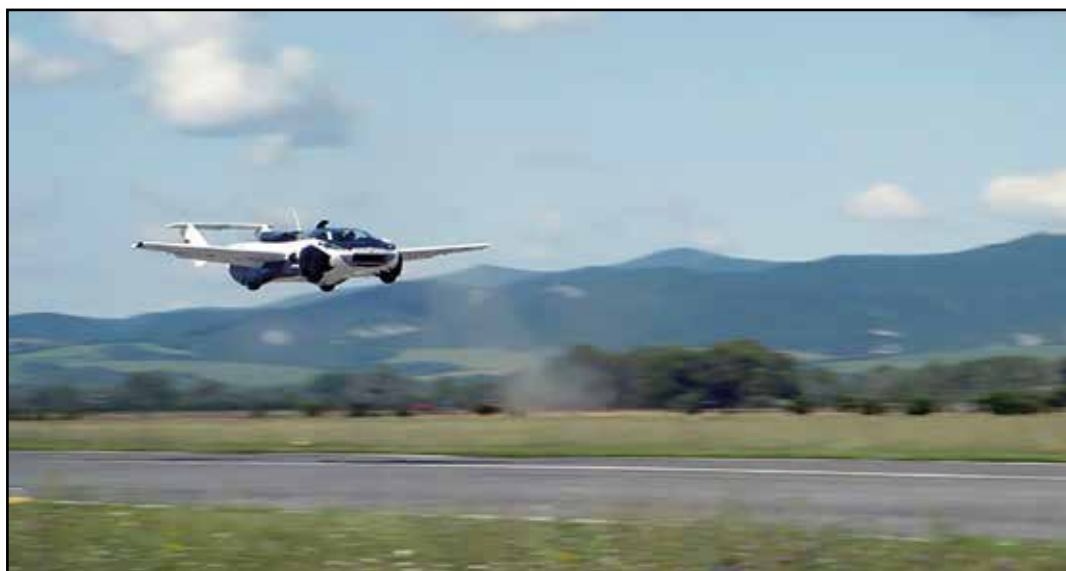
Above: The Klein Vision AirCar is a more orthodox looking aeroplane and a more orthodox looking car. It can fly at a top speed of 180mph and has a 600 mile flight range and a ceiling of 18,000ft.
