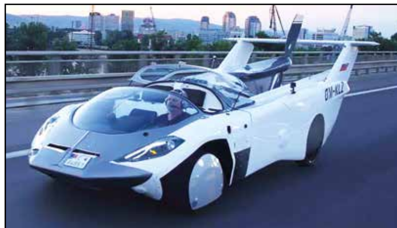
Above: The Klein Vision AirCar is a more orthodox looking aeroplane and a more orthodox looking car. It can fly at a top speed of 180mph and has a 600 mile flight range and a ceiling of 18,000ft.
